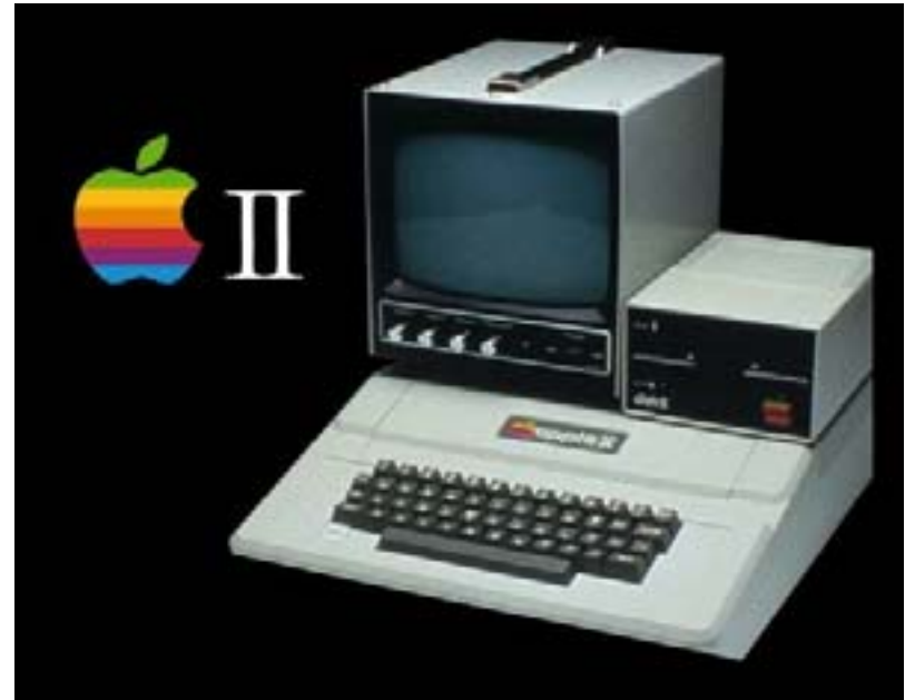
Apple II 1 MHz CPU, 48k RAM Data stored on audio cassette On sale June 1977 ($2,638)
